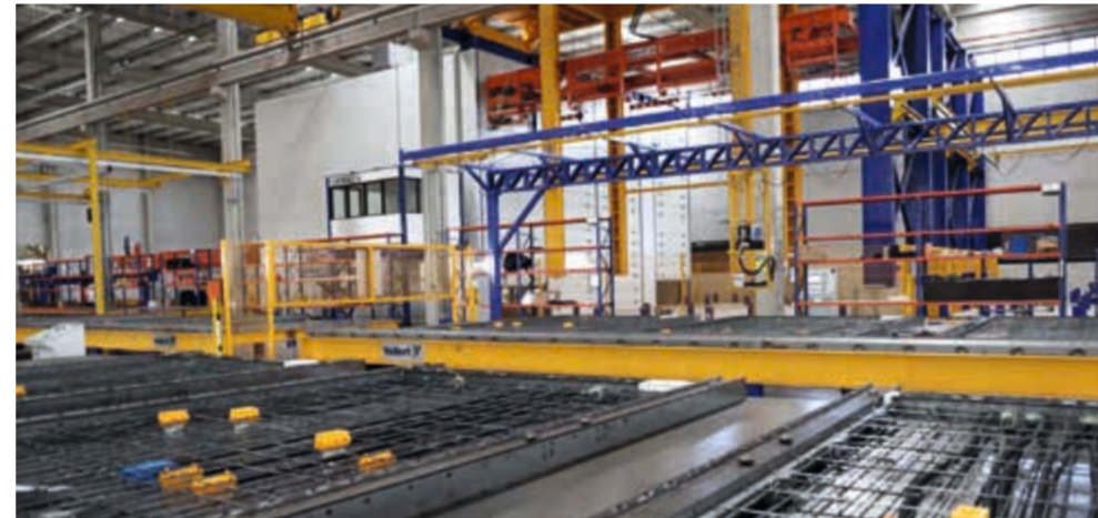
Robot-compatible SAS Standard automatic mould for solid elements (Image: Jonathan Campos / AEN)
