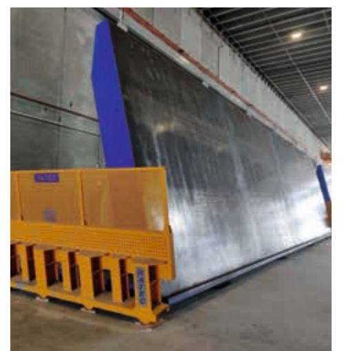
Hydraulic tilting table for prestressed elements
