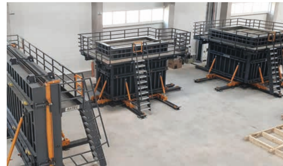
View of the factory with a vertical roof mould and two modular moulds
