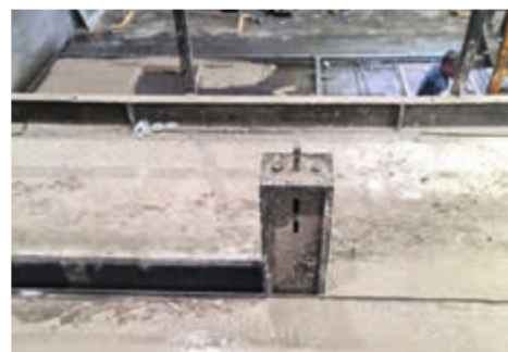
Laterally movable inner shuttering for battery moulds
