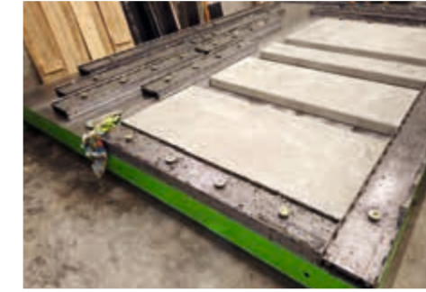
Shrinking formwork for double-sided concreting and robot operation
