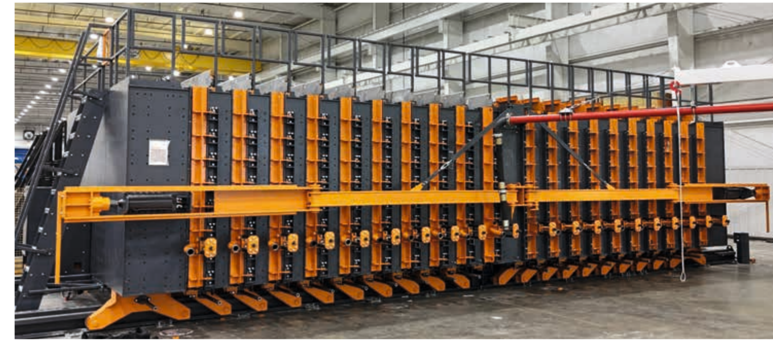
With 2 x 10 pockets, this is the largest battery mould that RATEC has ever installed
