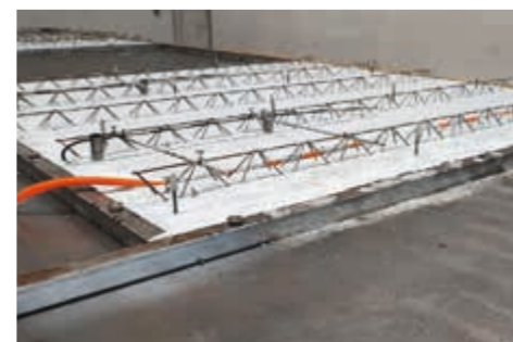
RT U60 Pro for girder slabs and double walls
