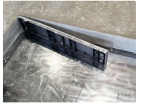
Side pieces for adjusting the size of the window frame
