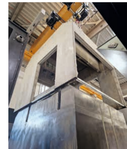
Finished station element
