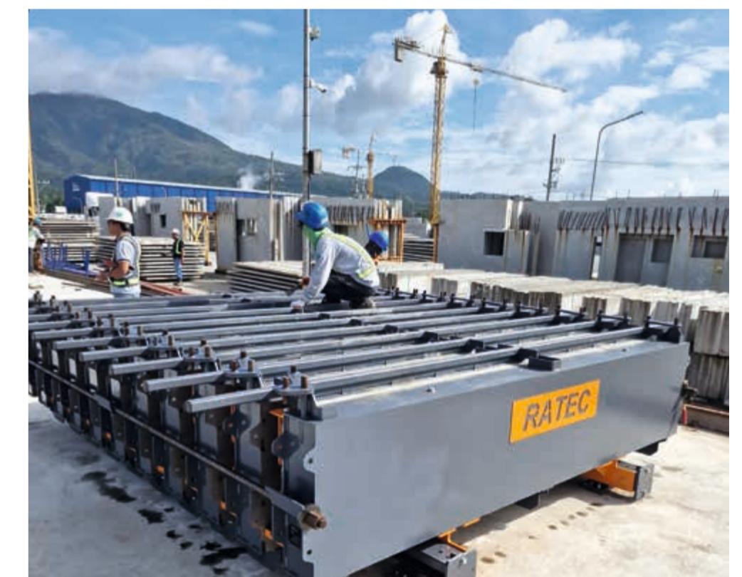
Battery system with ten pockets for walls approx. 2.7 metres long and 60 centimetres high
