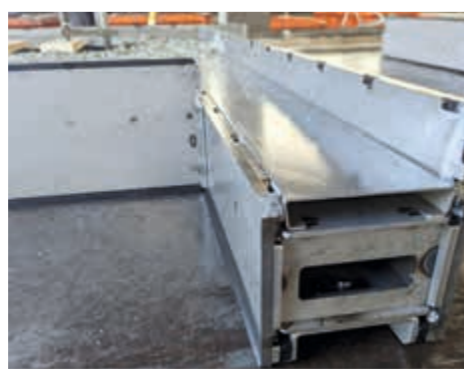
Rubber lips and cover plate protect against soiling
