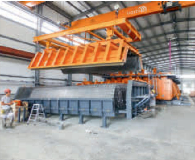
Example: Roof moulds for upcrete®, filling from below
