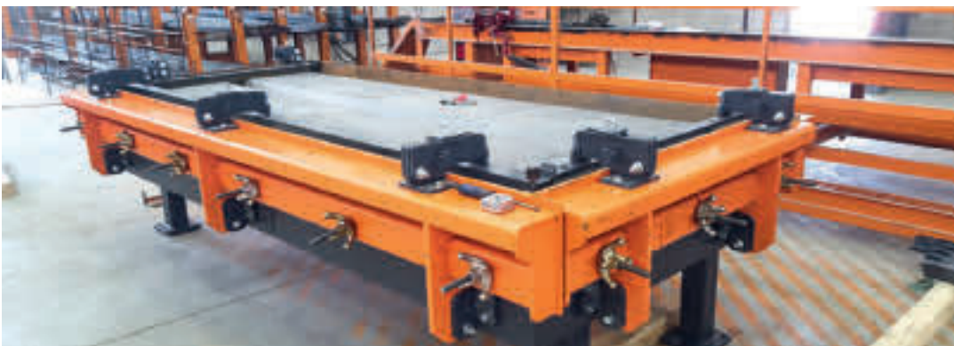
Moulds for a flat roof with contouring at the bottom for filling from above
