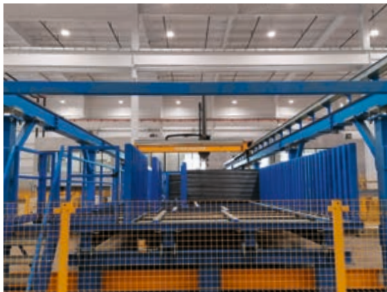
Completely automated formwork logistics from storage retrieval and placing up to cleaning
