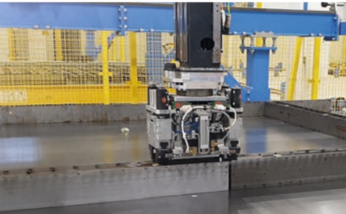
Completely automated formwork logistics from storage retrieval and placing up to cleaning
