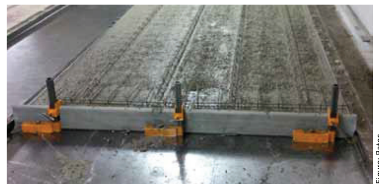
The Speedy GF-5 can be placed lengthwise or crosswise to the concrete element
