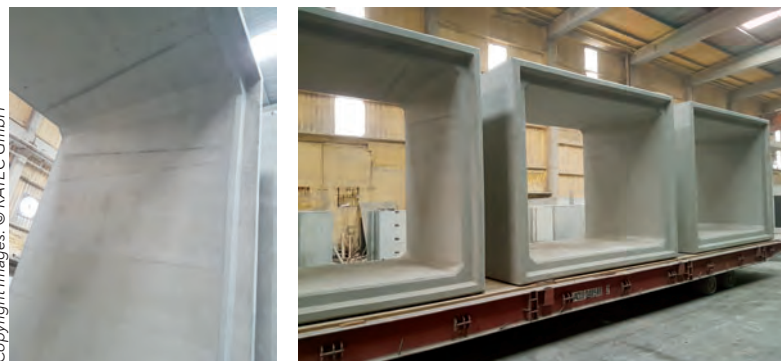
Box culverts that were produced by pumping the concrete from below
