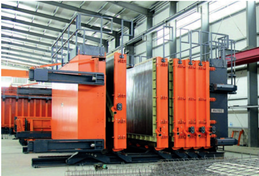
Example of an opened battery mould – special moulds that form the element geometry were clamped in the "pockets" of the battery for the façade elements of the Palazzo Italia.
