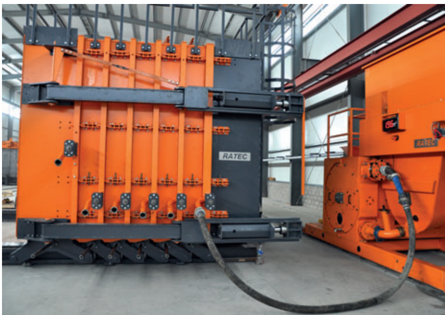
Example of a battery mould with connected upcrete pump
