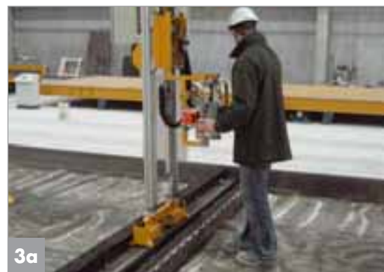
Shuttering handling crane during shuttering
