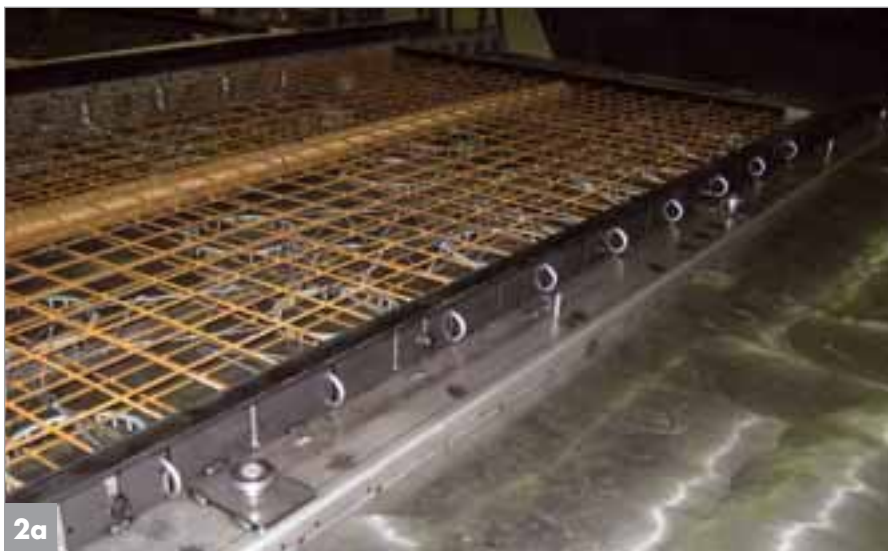
Flexible shuttering systems with connecting reinforcement
