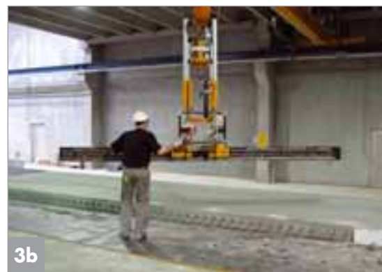
Shuttering handling crane during de-shuttering
