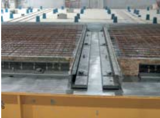
Fig. 4 Customized steel modules in various designs can be used to form the casting joint.
