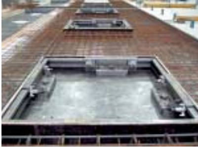
Fig. 3 Simple formwork solutions also for door and window openings.
